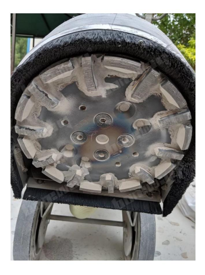
10 inch Diamond Grinding Disc. Metal bond diamonds have high strength, excellent wear resistance, and a low friction coefficient.
