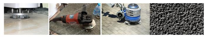
**Concrete Alloy Bush Hammer Roller** can be adjusted with our bush hammer through adjustment of spring elasticity on the bush hammer, or through the pressure of the manual grinding machine.
