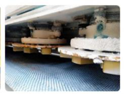
**Frankfurt Sharp Blasting Media Abrasives** is designed for marble calibration and rough grinding. This Frankfurt plate is designed with selected metallic powder and high concentration of diamond that gives good grinding power to calibrate and grind marble slab and tiles. With use of metallic plate, pressure of polishing head would be greatly decreased and longevity of abrasives stone would be greatly extended, i.e. metallic plate helps save both cost and energy.
