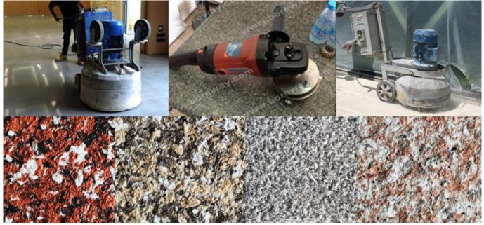
45 Teeth Alloy Granite Concrete Bush Hammered Tools Application Disc:
