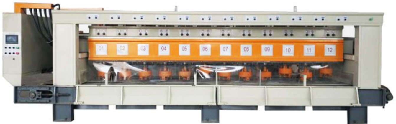
Automatic Bush Hammer Machine
