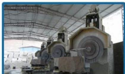
One is single size multi cutter, which all blade sizes in same thickness and diameter while the other is multi size multi cutter, two sizes or more different size diameter blades used together in one stone machine.
